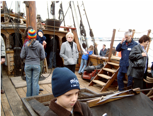
Fig. 22) Next to the completely open forecastle, the waist bulkhead for the half-deck with its two large open doors and four half-high window openings can only be accepted as charade. Being only several feet above the waterline even larger ships had closed doors and no windows in this bulkhead. This is complete fantasy.
